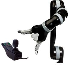
Fig. 3. MICO assistive robot and 3-axis joystick (Kinova).
