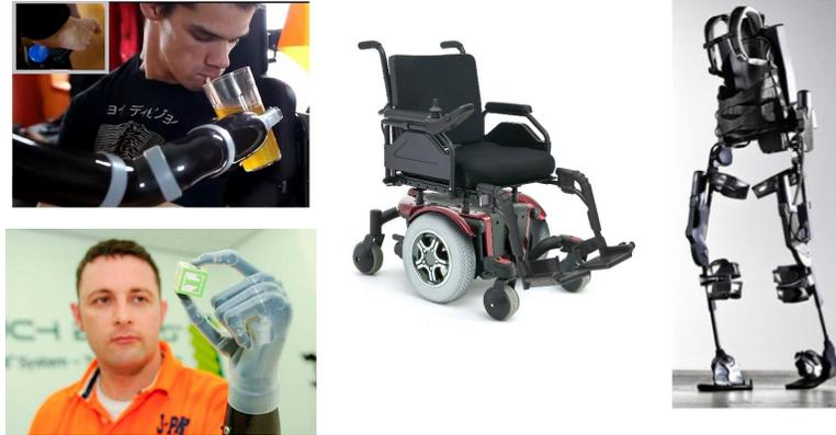
Figure 1. Examples of commercially available assistive machines. *Clockwise from top left:* The JACO wheelchair-mounted robotic arm from Kinova Robotics,<sup>7</sup> operated via a foot-controlled 3-axis joystick (inset). The Quantum 600 powered wheelchair from Pride Mobility,<sup>8</sup> that provides the base for our mobile robot platform (Fig. 2). The Ekso Hope lower limb exoskeleton from Ekso Bionics.<sup>9</sup> The i-limb ultra prosthetic hand from TouchBionics.<sup>10</sup>
