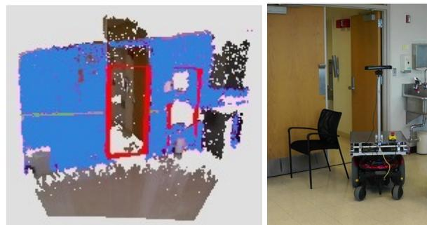
Figure 8. Autonomous doorway detection (red box) and traversal using only depth information from a Kinect and our autonomous doorway detection algorithm.<sup>84</sup>
