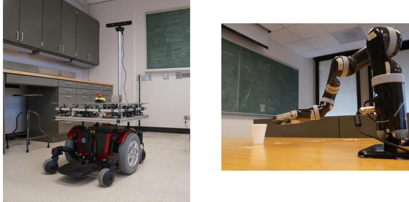
Figure 2. *Left:* Smart wheelchair platform under development in the *argallab*, which includes a ring of IR and ultrasonic sensors and a top-mounted Kinect RGB-D sensor. *Right:* The MICO robotic arm in our lab, a 6+1 DoF robotic arm (6 arm joints + 1 gripper), which observes the external world through a single Kinect sensor.
