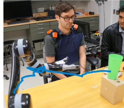
Figure 6. Proof-of-concept teleoperation of 2-D of the 6-DoF MICO robotic arm using the BMI (the remaining 4-D are fixed). Execution path in blue.
