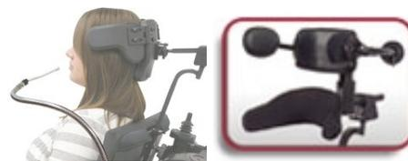
Figure 5. Examples of non-proportional control interfaces. *Left:* The Sip-N-Puff<sup>67</sup> issues commands by blowing and sucking on a straw. *Right:* A switch-based electronic head array with three proximity sensors.<sup>68</sup>
