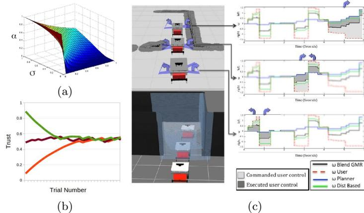
Figure 4. Preliminary studies with control sharing. (a) Blending parameter  $\alpha$  is a function of trust that informs  $\alpha$ . (b) Evolution of a measure of trust that informs  $\alpha$ . (c) Snapshots of stress testing shared control.<sup>36</sup> Plots show user-commanded rotational speeds (blue arrows), and amount of executed (dark gray) and unexecuted (light gray) user-commanded control. Image from Goil, *et al.*, 2013.<sup>36</sup>
