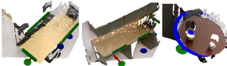
Figure 9. Autonomous docking location detection (green and blue circles) on example docking structures (left to right: rectangular conference table, desk, circular table). On the circular table, the docking location is anchored to the detected place setting (bowl). Image from Jain, *et al.*, 2014.<sup>85</sup>
