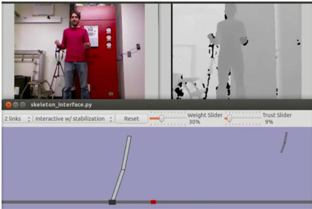
Fig. 1. An example of software-supported motion direction. A person (upper left) demonstrates motion using the Kinect sensor (upper right) to control a virtual double inverted pendulum (bottom). The person’s motion is augmented by the synthesized feedback controller so that the double inverted pendulum motion projects back to a stable, feasible motion.
