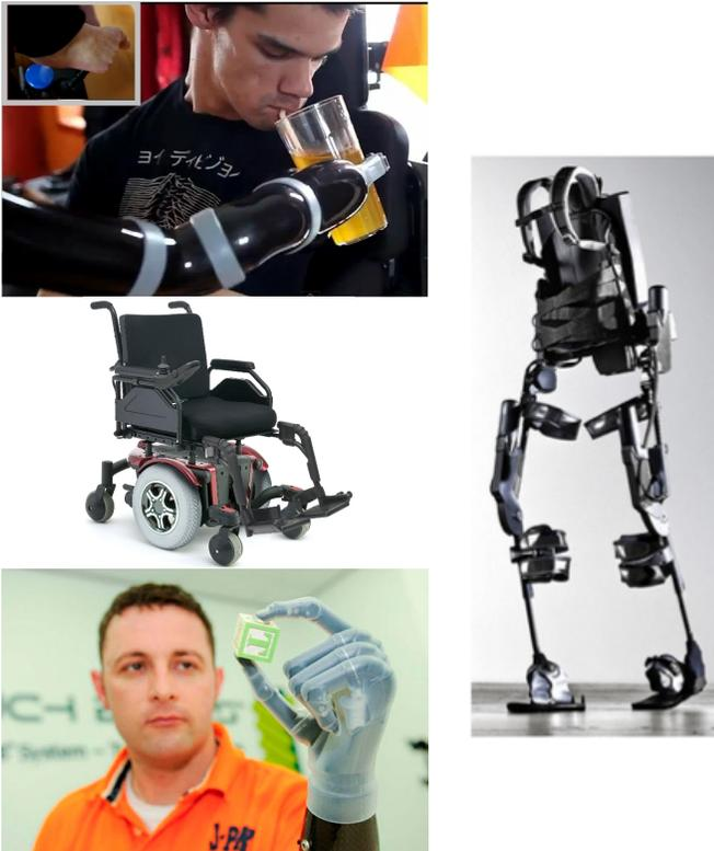
Fig. 1. Examples of commercially available assistive machines. *Clockwise from top left*: The JACO wheelchair-mounted robotic arm from Kinova Robotics [1], operated via a foot-controlled 3-axis joystick (inset). The Ekso Hope lower limb exoskeleton from Ekso Bionics [2]. The i-limb ultra prosthetic hand from TouchBionics [3]. The Quantum 600 powered wheelchair from Pride Mobility [4], that provides the base for our mobile robot platform (Fig. 2).
